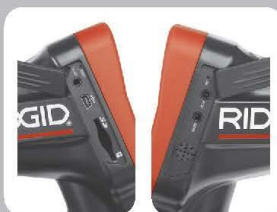
TV Out, USB, SD Card Storage Speaker, Mic, Head Set Jack, AC Power Input
