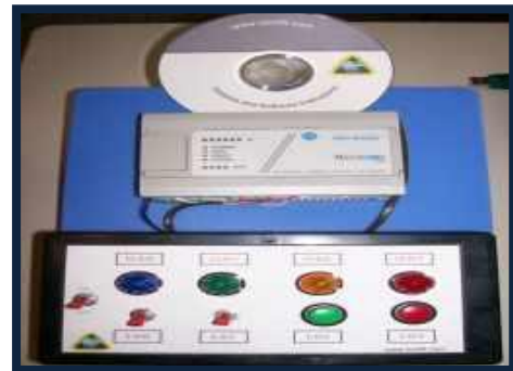
Allen Bradley Micrologix 1000 Simulator (Digital)
