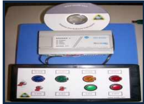
Allen Bradley Micrologix 1000 Simulator (Digital)
