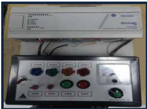
Allen Bradley Micrologix 1000 Simulator (Analog)
