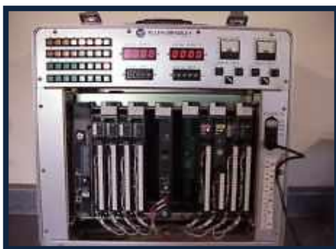
Allen Bradley WS5610 PLC Simulator PLC5
