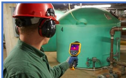
Infrared thermography technique which is non-contact, nondestructive test method uses an infrared imaging to detect, display and record thermal patterns and temperature across the surface of an object.
