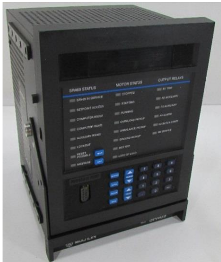
GE Multilin Relay 469 Simulator
